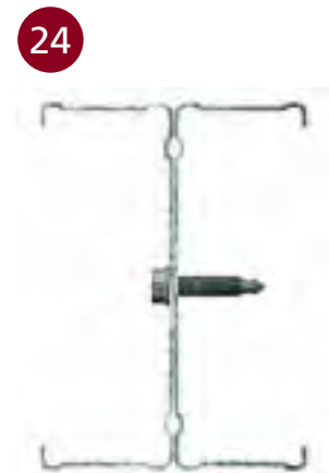
■ TYPICAL STUD FRAMING SECTIONS
