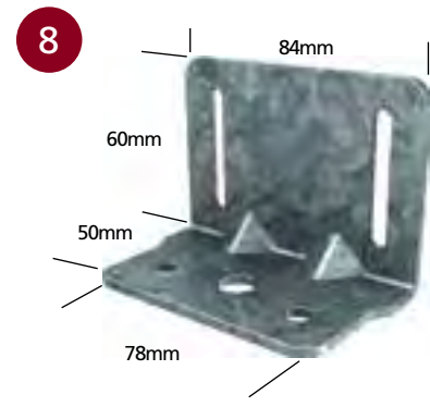
■ 203 SLOTTED JAMB HEAD BRACKET
