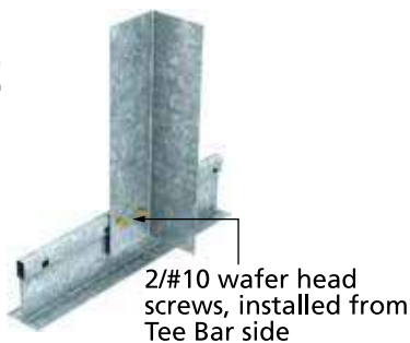
WAH/SA12 secured to tee web
