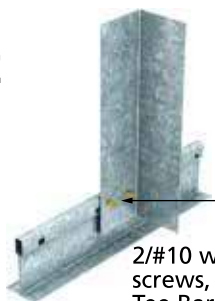
WAH/SA12 secured to tee web
